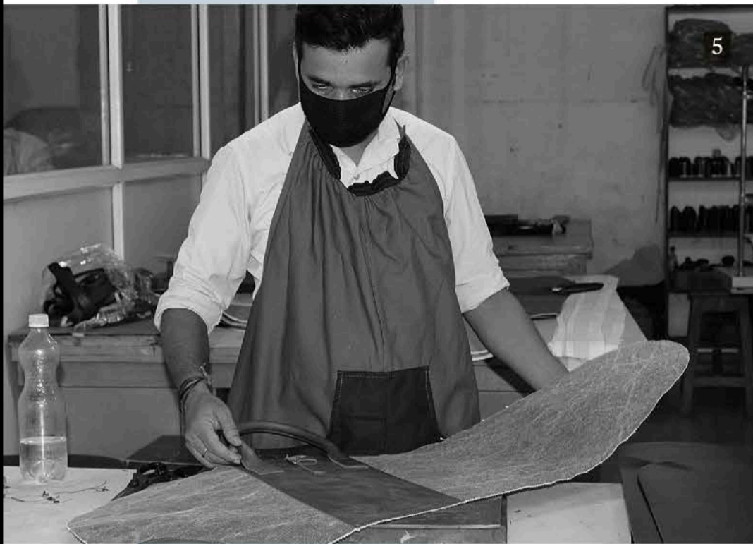
5. The outer layer of canvas and leather sits on top of a multi-layered shell in which rubber, unbreakable plastic, foam and paper composite all form part of a unique protection system
